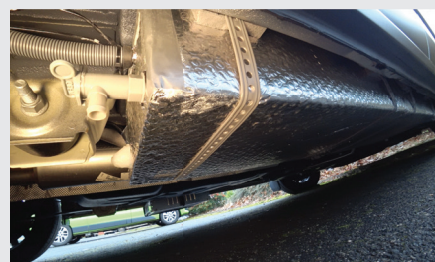
Heating and insulating the 'van water tanks helps to prevent them freezing
