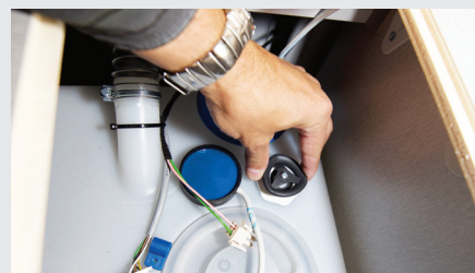
Most motorhome fresh-water tanks have a drain-down valve at the top
