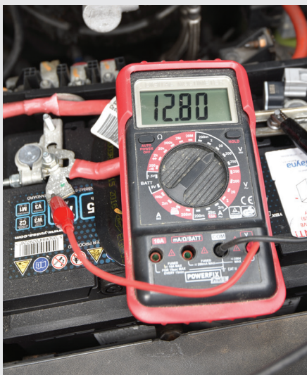
You can easily check if your charger also tops up the vehicle battery by using a multimeter set to volts – the voltage will increase when hooked up if it's receiving any charge
