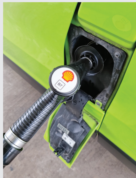
Diesel engines have had 7% biofuel in them for some years now – it's advisable to store them in winter with a full tank
