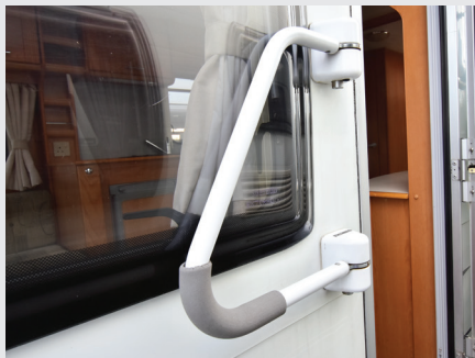
The habitation door in a coachbuilt 'van could tempt thieves, but a locking 'D' handle can provide additional security
