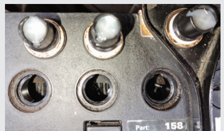
Lead plates must be immersed. If not, you'll need to add deionised water (not tap water, which will damage the cells)
