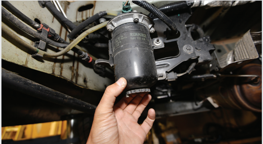
Buy your diesel after mid-October to ensure that you lay up your motorhome with winter diesel and avoid problems with waxy crystals blocking fuel filters such as this
