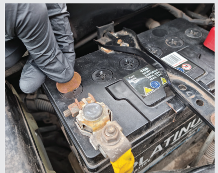
To top up the fluid in a lead acid battery, remove the cell cap with a coin. Always wear gloves and eye protection for this
