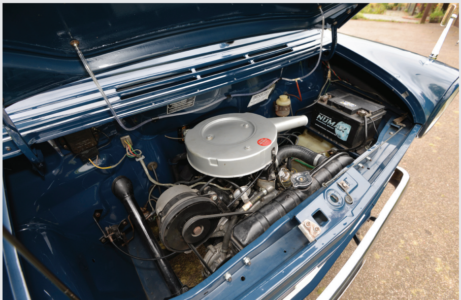
Older vehicle engines – pre-2000 and anything with a carburettor – should only be operated on E5 super-unleaded fuel, to avoid potential problems with biofuel
