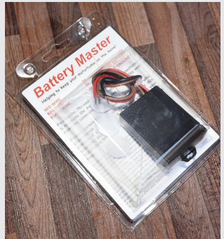
The Battery Master is a simple way to have your vehicle battery topped up automatically by the leisure batteries
