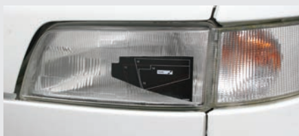
Headlight deflectors on British vehicles are mandatory in countries that drive on the right-hand side of the road
